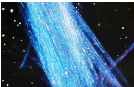
Figure D.52 — Richterite/winchite asbestos in 1.630 RI liquid viewed in dispersion staining, fibres at extinction position.
