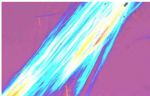
Figure D.49 — PLM micrograph of richterite/winchite asbestos in 1.630 RI liquid, crossed polars with 550 nm retardation plate.
