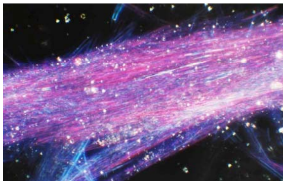
Figure D.51 — Richterite/winchite asbestos in 1.630 RI liquid viewed in dispersion staining, fibres at extinction position.
