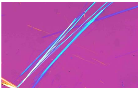
Figure D.23 — PLM micrograph of NIST SRM 1867 tremolite in 1.625 RI liquid, crossed polars with 550 nm retardation plate.
