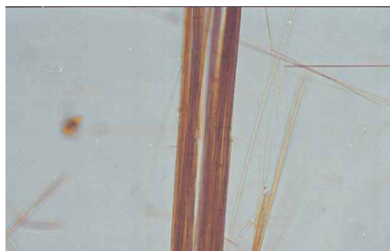
Figure D.10 — Heated amosite in 1.680 RI liquid viewed in plane polarized light, fibre length parallel to polarizer vibration direction.
