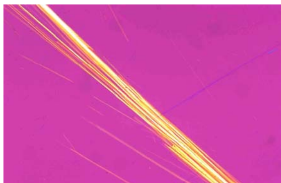
Figure D.32 — PLM micrograph of NIST SRM 1867 anthophyllite in 1.630 RI liquid, crossed polars with 550 nm retardation plate.
