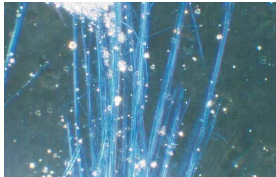
Figure D.4 — NIST SRM 1866 chrysotile in 1.550 RI liquid viewed in dispersion staining, fibre length normal to polarizer vibration direction
