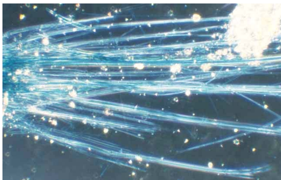
Figure D.15 — NIST SRM 1866 crocidolite in 1.700 RI liquid. Dispersion staining, fibre lengths parallel to polarizer vibration direction.
