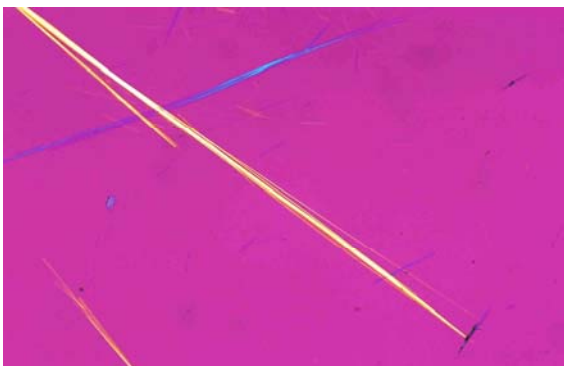
Figure D.28 — PLM micrograph of NIST SRM 1867 actinolite in 1.630 RI liquid, crossed polars with 550 nm retardation plate.
