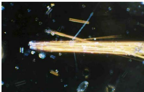
Figure D.47 — IOM anthophyllite in 1.605 RI liquid viewed in dispersion staining, fibre lengths parallel to polarizer vibration direction.
