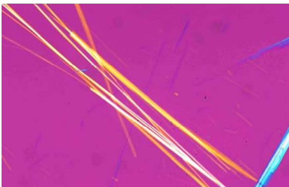
Figure D.24 — PLM micrograph of NIST SRM 1867 tremolite in 1.625 RI liquid, crossed polars with 550 nm retardation plate.
