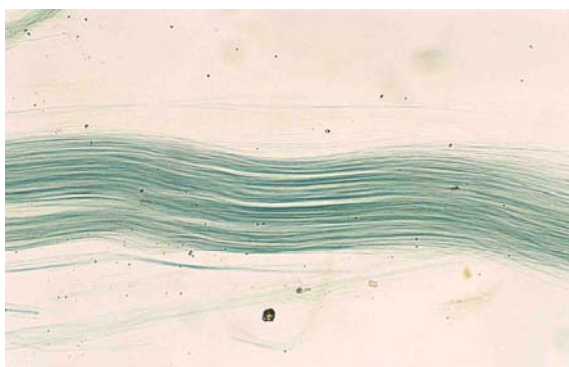
Figure D.43 — IOM actinolite in 1.640 RI liquid in plane polarized light, fibres parallel to polarizer vibration direction.
