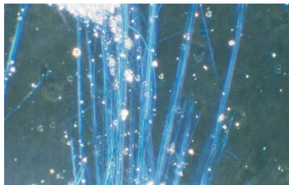
Figure D.16 — NIST SRM 1866 crocidolite in 1.700 RI liquid. Dispersion staining, fibre lengths normal to polarizer vibration direction.
