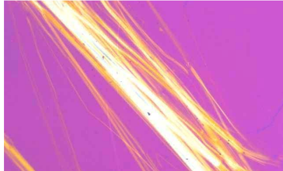
Figure D.2 — PLM micrograph of NIST SRM 1866 chrysotile in 1.550 RI liquid, crossed polars with 550 nm retardation plate
