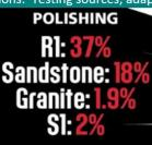
The average percentage of CRYSTALLINE SILICA in respirable dust emissions when polishing
