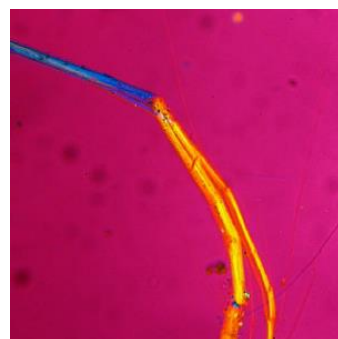
Figure 5: Rock 1 fibers 1.550 RI liquid, ~100x Cross-Polarized with 530nm waveplate.
