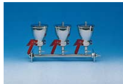
Figure 4: Multiple Vacuum Filtration Apparatus
