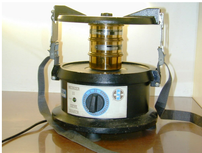
Figure 3 Configuration of 3” diameter sieves on the sieve shaker (Note: does not show 19mm sieve that would be on top)
